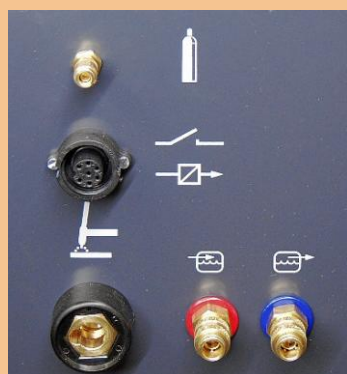
Connection panel - with water cooling.
